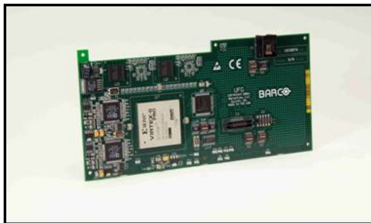
Figure 1.2: FLEXIVISION III Universal Frame Grabber Module
