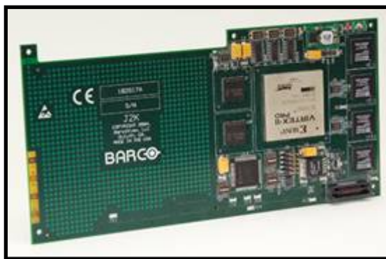
Figure 1.3: FLEXIVISION III JPEG 2000 Module
