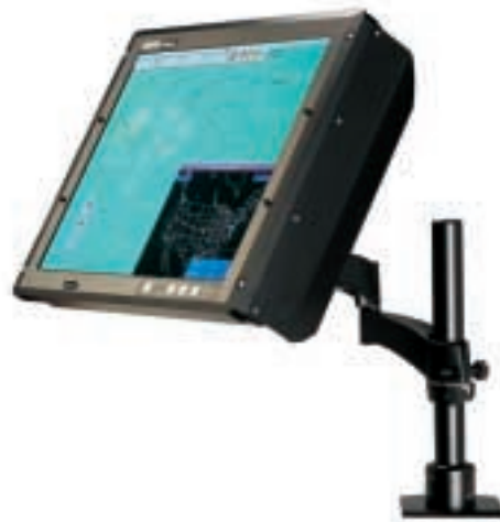
Barco's APA functionality avoids image artifacts as it automatically locks the LCD sampling clock to the (drifting) graphics generator pixel frequency
