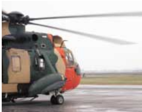
Barco's 20.1" rugged LCD displays have been integrated into several helicopter programs, including the Royal Navy's fleet of SeaKings. The airborne environment of the SeaKing is one of the most severe rotary wing platforms.
