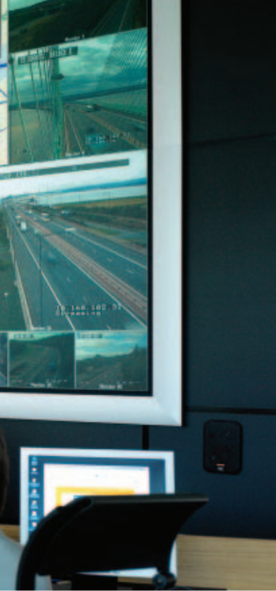
Barco OverVIEW CDR67-DL display modules in a 4 x 2 configuration controlled by the ARGUS graphical controller and managed by the APOLLO software.
