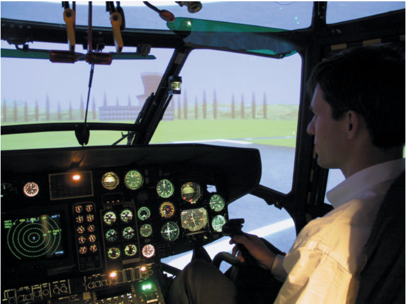
Figure 9: Helisim, France; Barco Genesys III Calligraphic Technology for Level D Full Flight Simulation
