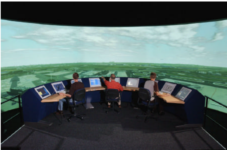
Figure 1: Three channel tiled display system used for Air Traffic Control (ATC) simulation Copyright 2002, National Aerospace Laboratory, Amsterdam, The Netherlands
