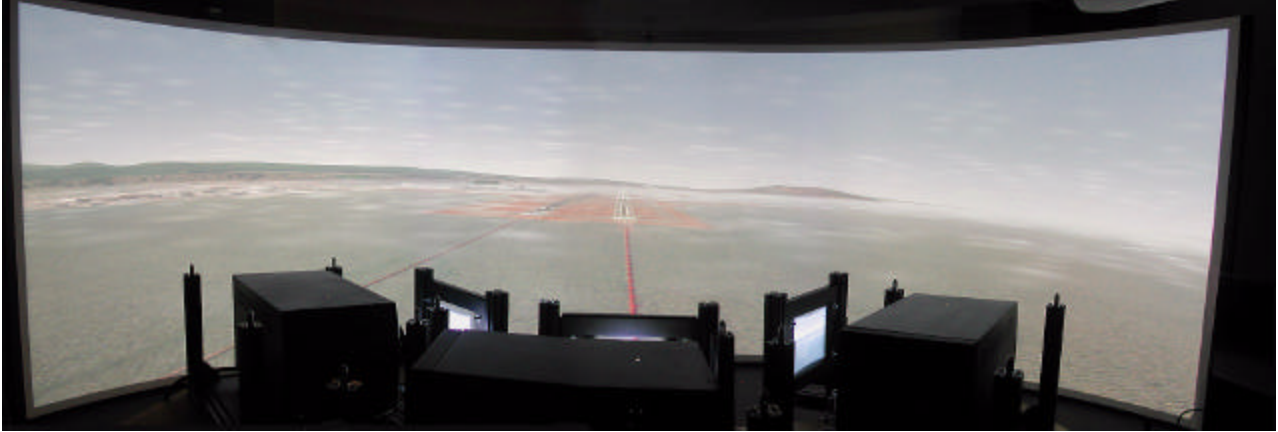
Figure 9: Helisim, France; Barco Genesys III Calligraphic Technology for Level D Full Flight Simulation
