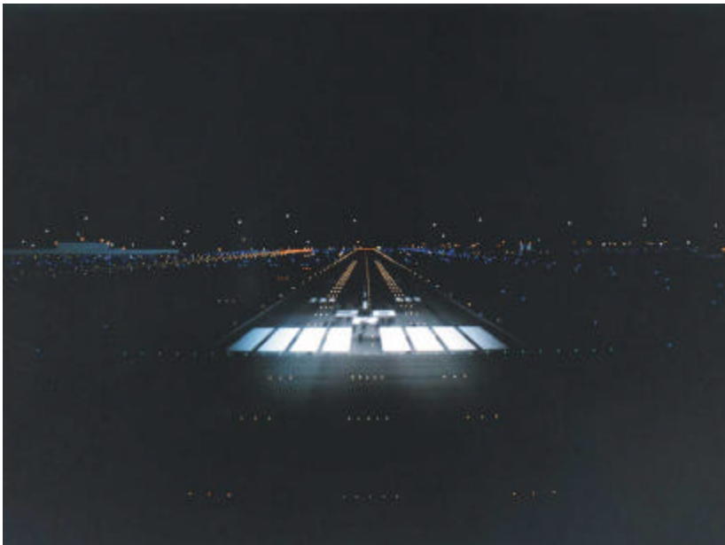
Figure 3: Typical Level D simulator image using both raster and calligraphic scanning techniques.
