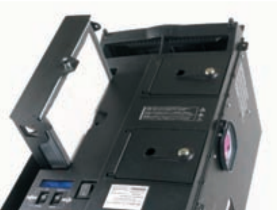
A dust filter keeps the electronics and lamps clean.
