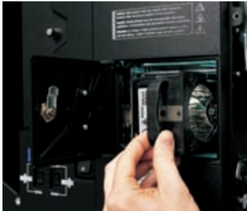
The lamp can be hot-swapped without image loss and without opening the system.
