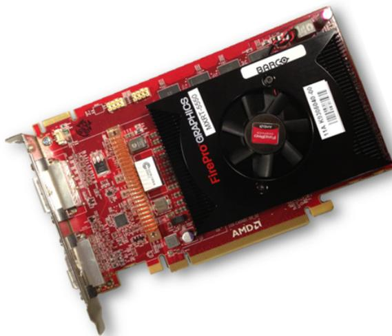
The board features 2 DVI connectors, providing a solid solution for upgrades.
