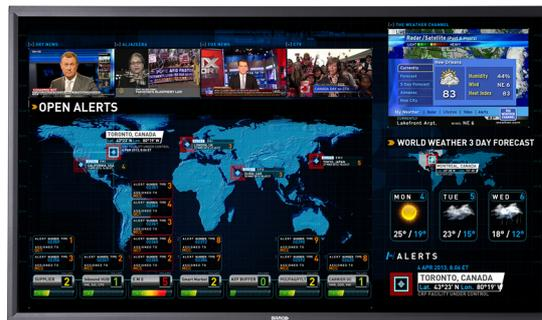
The LDX-58 RL is a large-screen LED-backlit personal workstation display, featuring a 58-inch LCD panel (16:9) with Quad HD resolution (3840 x 2160). It was designed for collaborative decision-making, combining a very high resolution with excellent contrast ratio, high brightness, and a wide viewing angle.
