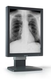
The high-grade Coronis 5MP display system offers unsurpassed film-like images with ultra-high resolution, luminance and contrast. The 21.3" LCD provides unequaled image quality without pixelization, a wide viewing angle and perfect geometry.
